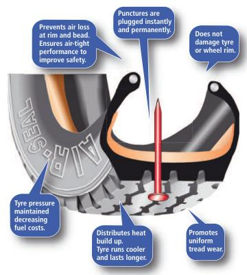
As the tyre rotates, the product spreads evenly over the inside surface. Immediately a puncture occurs, the air pressure in the tyre forces millions of fibre particles and fillers suspended in the sealant to interlock to form a plug which prevents any further air loss. This action will be completed within two or three revolutions of the wheel. This is a mechanical process not a chemical reaction.
